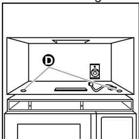
4. Hold microwave hood combination in place with one hand. Pull hook **E** to release microwave hood from mounting plate. If grille cannot be removed (per instructions in step 2.), insert a thin looped wire or similar tool through an opening in grille to pull hook.
